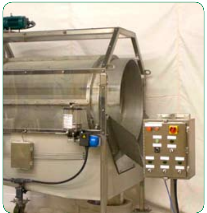
Drumscreen Monster includes an automated controller. JWCI offers an optional auto-lube system & variable frequency drives.
