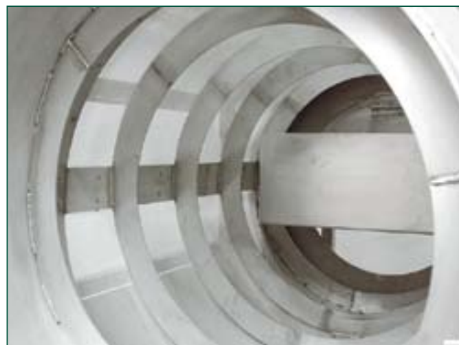
Sludge is distributed evenly across the continuous band of woven wire or wedge wire mesh panels in the screening zone.
