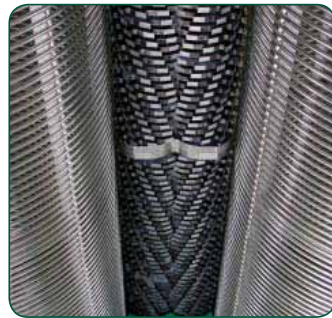
Coil screening drums
